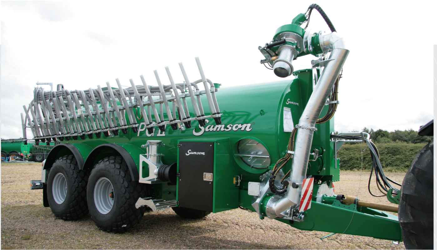
Double-articulated SAP arm (SAP2) with or without pump
