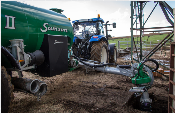
Direct filling from underground storage of slurry
