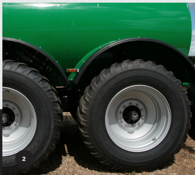
The large wheels reduce rolling resistance.
