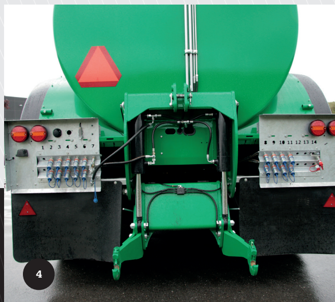
Hydraulic couplings are located where they are easily accessible.
